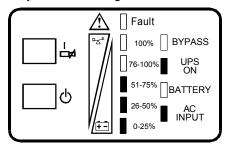
Figure 1- Normal Mode Operation at 51-75% loading
